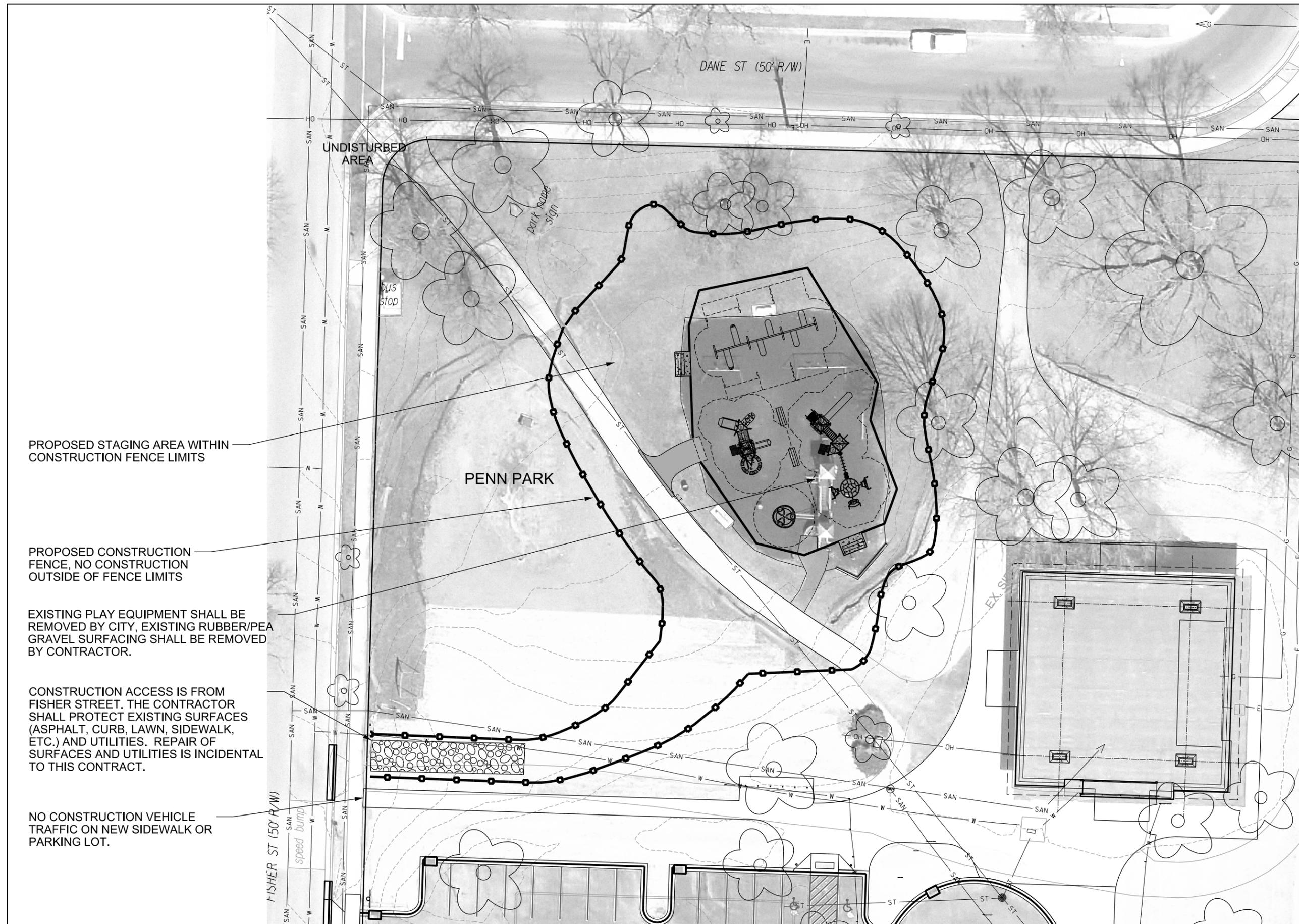
PROPOSED STAGING AREA WITHIN CONSTRUCTION FENCE LIMITS
